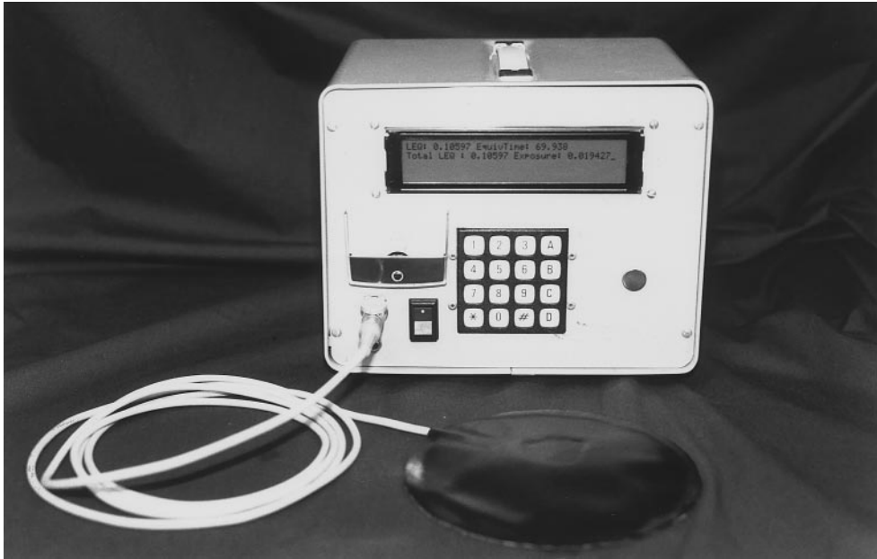
Figure 5. Digital vibration dosimeter and three-axis accelerometer seatpad.
